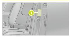
The tyre pressure table is located on the front of left B pillar 1.
