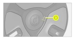
Insert the hook into the wheel trim cover hole and pull it outward to remove the wheel trim cover.
