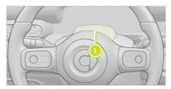
The Driver Monitoring System camera 1 is located on the steering column at the rear of the steering wheel.
