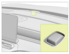
The light sensor is located in the centre of the instrument panel, and the automatic wipers/automatic headlamp/automatic climate control controls the corresponding functions through this sensor.
