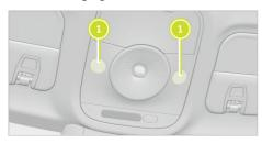
**ON/OFF:** touch or press the reading light depending on the vehicle configuration. Depending on the vehicle configuration, press and hold the physical switch of the
