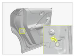
Turn the door lock in the direction of the arrow until it stops. The door will be locked once closed.
