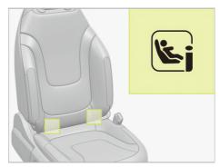
Before every trip, make sure that the ISO-FIX/i-Size child restraint system is engaged correctly in both anchor points on the seat.
