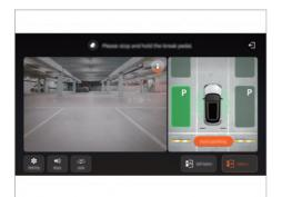
When the vehicle speed is below 30 km/h, tap to enter the application interface and tap to enter the Automatic Parking Assist interface, or press the button to enter the Automatic Parking Assist interface.
