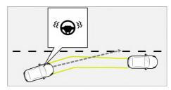
If the driver does not actively control the vehicle and the system detects that the vehicle is deviating from the current lane, the Lane Departure Prevention will actively request steering to help the vehicle return
