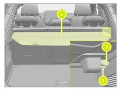
To remove: pull out and remove the boot separator 1.
