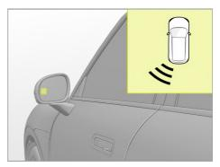
If Door Opening Warning detects the target and a collision risk when the door is open, the system will flash the outside rearview mirror indicator and issue a sound warning, and the driver information display will show the corresponding object warning prompt.
