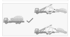
When the wheels rotate, the front and rear E-motors of the vehicle can generate electric energy. It is recommended to transport the vehicle with flatbed trailers or similar transport vehicles. As shown in the figure above, make sure that the tyres cannot move during transportation.
