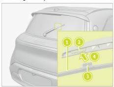
Place the wiper blade 1 onto the bracket of wiper arm 2 through the 2 lugs 3.
