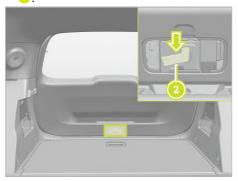
3. Press the unlock switch 2 and the liftgate unlocks.
