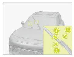
3. Hold the wiper arm with one hand, press the clip inward along the direction of the arrow 1, and pull the blade out along the direction of the arrow 2 with the other hand.
