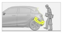
When the vehicle detects the keyfob, you can open, close, or stop the liftgate by kicking below the rear bumper.
