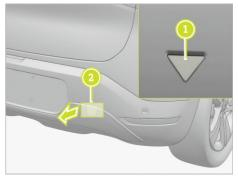
Press the lower point of the triangular indicator 1 inward to remove the tow bar cover 2.
