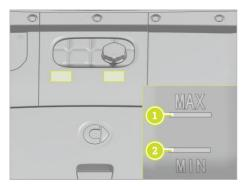
If the coolant level is lower than the marked position 2, inspect or top up coolant at a smart Authorized Service Partner
